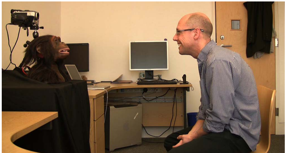
Fig. 3 The experimental setup. A participant sits in a chair facing the robot, about one meter away from it. The camera and chair position remain fixed across all participants
