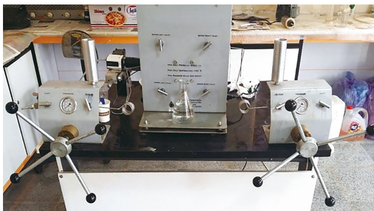
Fig. 3 A schematic diagram of a VIT-6000 apparatus used to measure IFT and contact angle
