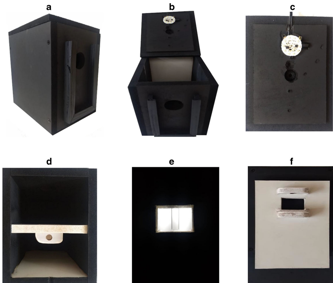
Fig. 1 Apparatus made for the determination of phenols and antioxidants in foods. Data collection box: overview front (a), internal view (b), LED cap (c), and photo test tube holder (d), window (e)
