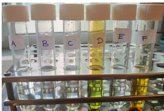
Fig. 1 Photo of tamarind samples after analysis with six different microwave digestion methods. a 8 mL HNO 3 , b 6 mL HNO 3 + 2 mL H 2 O 2 , c 6 mL HNO 3 + 2 mL HCl, d 12 mL HNO 3 , e 8 mL HNO 3 + 4 mL H 2 O 2 , f 8 mL HNO 3 + 4 mL HCl
