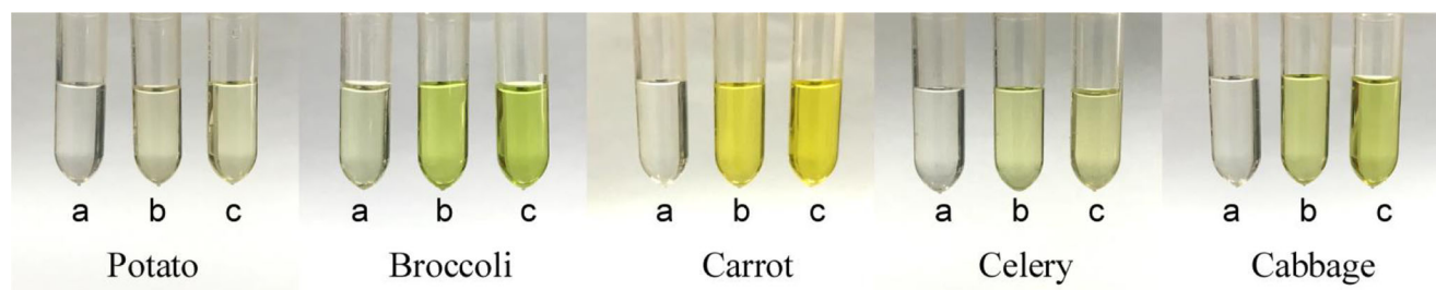
Fig. 2 Pictures of five matrices extracts after cleanup with MWCNTs (a), PSA (b), and no cleanup (c)
