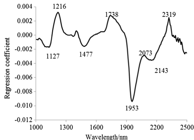
Fig. 3 Selection of optimal wavelengths corresponding to the large values of regression coefficients of the raw-PLSR model in the spectral range II
