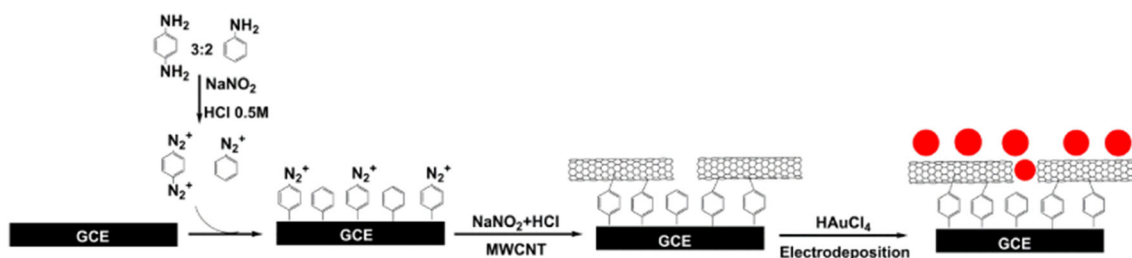
Fig. 2 Schematic representation of SWCNT and AuNP assembly on GCE
