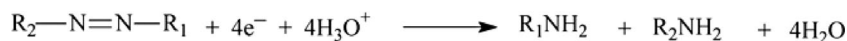
Scheme 2 Reduction mechanism for the SY and TT colorants at the Fe 3 O 4 @SiO 2 /MWCNTs-CPE surface
