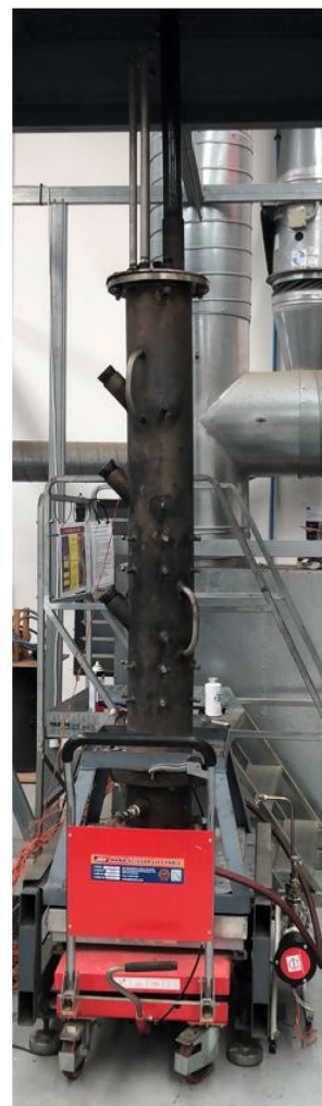
Fig. 3 Combustion mode: Laboratory-scale fixed-bed biomass combustor
