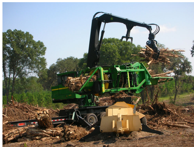
Fig. 4 A John Deere slash bundler. Photo: Mitchell
