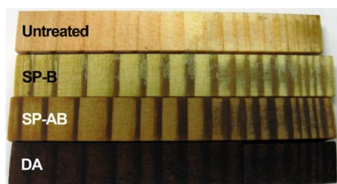
Fig. 1 Images of Douglas fir wood strips before and after dilute acid (DA) and SPORL pretreatments at different initial pHs (SP-B: pH=4.5; SP-AB: pH=2.0)
