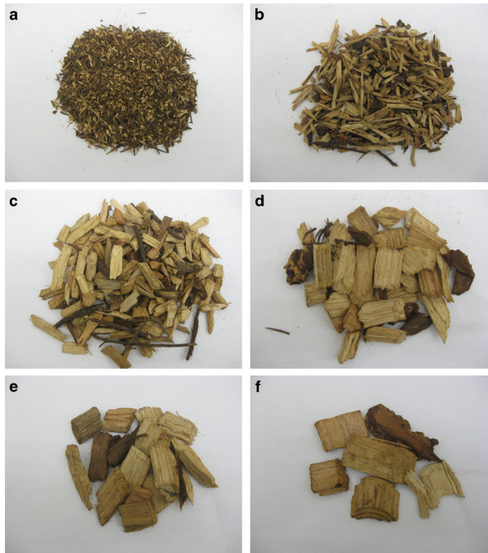
Fig. 1 Images of selected sieving fractions of the Douglas-fir forest residues. a Fraction I, <3.2 mm; b fraction III, 4.8–6.4 mm; c ) fraction V, 9.5–12.7 mm; d ) fraction VII, 15.9–19.1 mm; e ) fraction IX, 22.2–25.4 mm; f ) fraction XII, >31.8 mm
