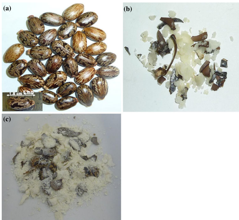
Fig. 2 Castor seeds before and after biodiesel production. a Intact castor seeds before biodiesel production with length of 1.8 cm. b Broken castor seeds before biodiesel production. The size of shell is around 3–15 mm, and the size of the white core containing the oil is around 0.5–5 mm. c Broken castor seeds with SrO after biodiesel production by direct transesterification using microwave
