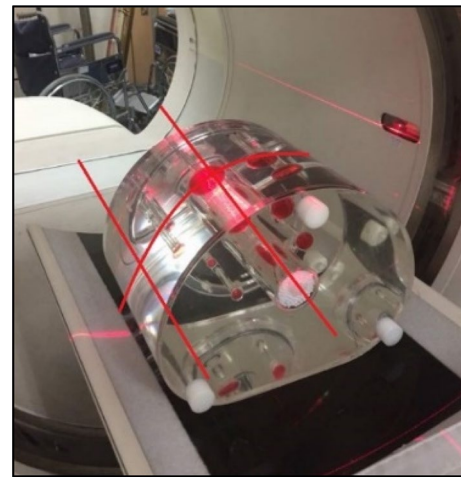
Fig. 1 NEMA2012/IEC2008 phantom positioning on GE Discovery ST PET–CT
