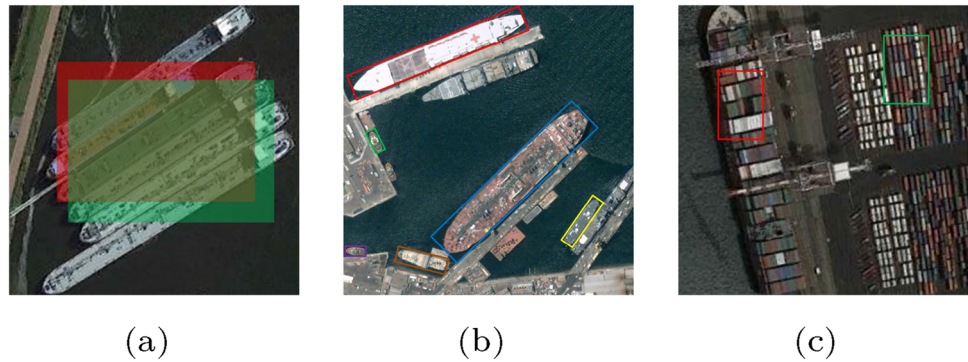
Fig. 1 Difficulties in remote sensing ship detection. (a) Dense arrangement. (b) Variable direction. (c) Complex background
