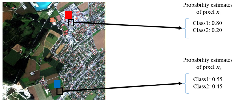
Fig. 2 Example of using probability estimates of one pixel to determine the classification reliability
