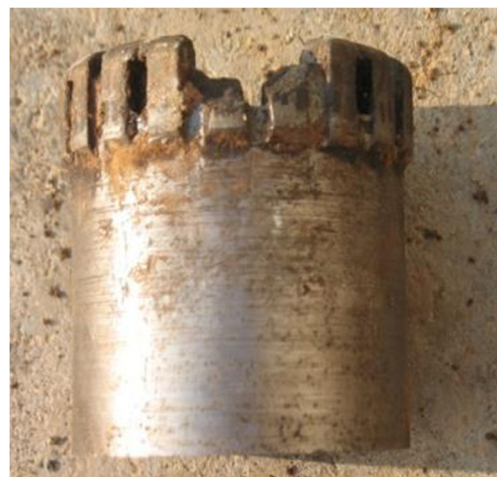
Fig. 10 The picture of the broken drill bit
