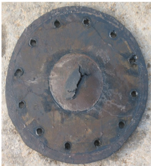
Fig. 12 Broken pump pad
