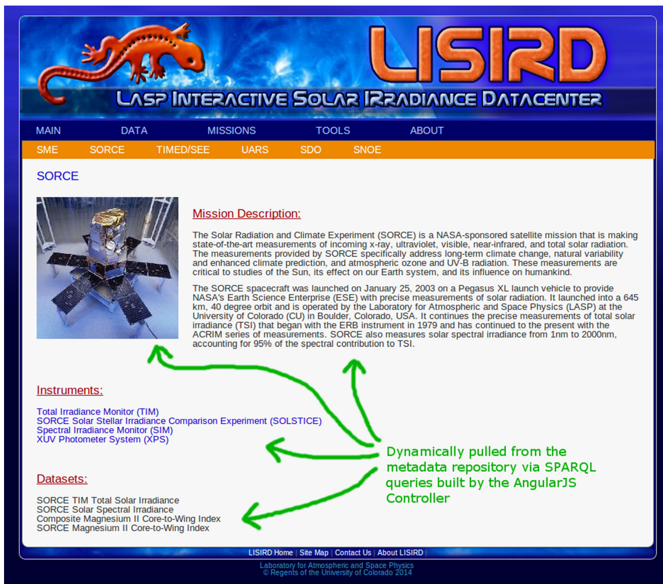
Fig. 3 A dynamic mission page created by an AngularJS controller. This page was created by requesting the URL “ http://www.example.edu/lisird/missions/sorce ”. the AngularJS controller looks for the token appearing
