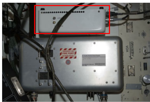
Fig. 1 The Air Quality Monitor (AQM)/Station Development Test Objective (SDTO) is shown (circled in red) attached to the Crew Health Care System (CHeCS) rack located in the center of the International Space Station's LAB module. The Volatile Organic Analyzer (VOA) was still in the rack just to the right of the AQM power supply (large silver box)
