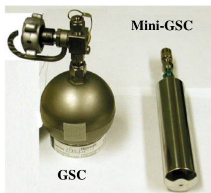
Fig. 3 Archival Air Samplers: Grab Sample Container (GSC), which is Summa™-treated stainless steel (approximate volume of 300 ml), and Mini-Grab Sampler Container (mini-GSC), which is Silonite®-treated stainless steel (volume of approximately 200 ml)
