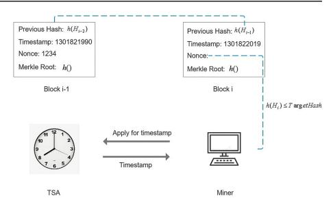
block to other nodes. Repeating this process, again and again, the timestamp of the node and the block will be more accurate than before. Selfish mining and time jacking will be more difficult for its attack window will be smaller. A high-level description is presented in Fig. 2.
