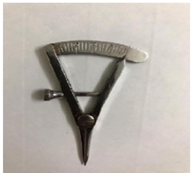
Fig. 1 Castroviejo caliper to measure the size of perforation
