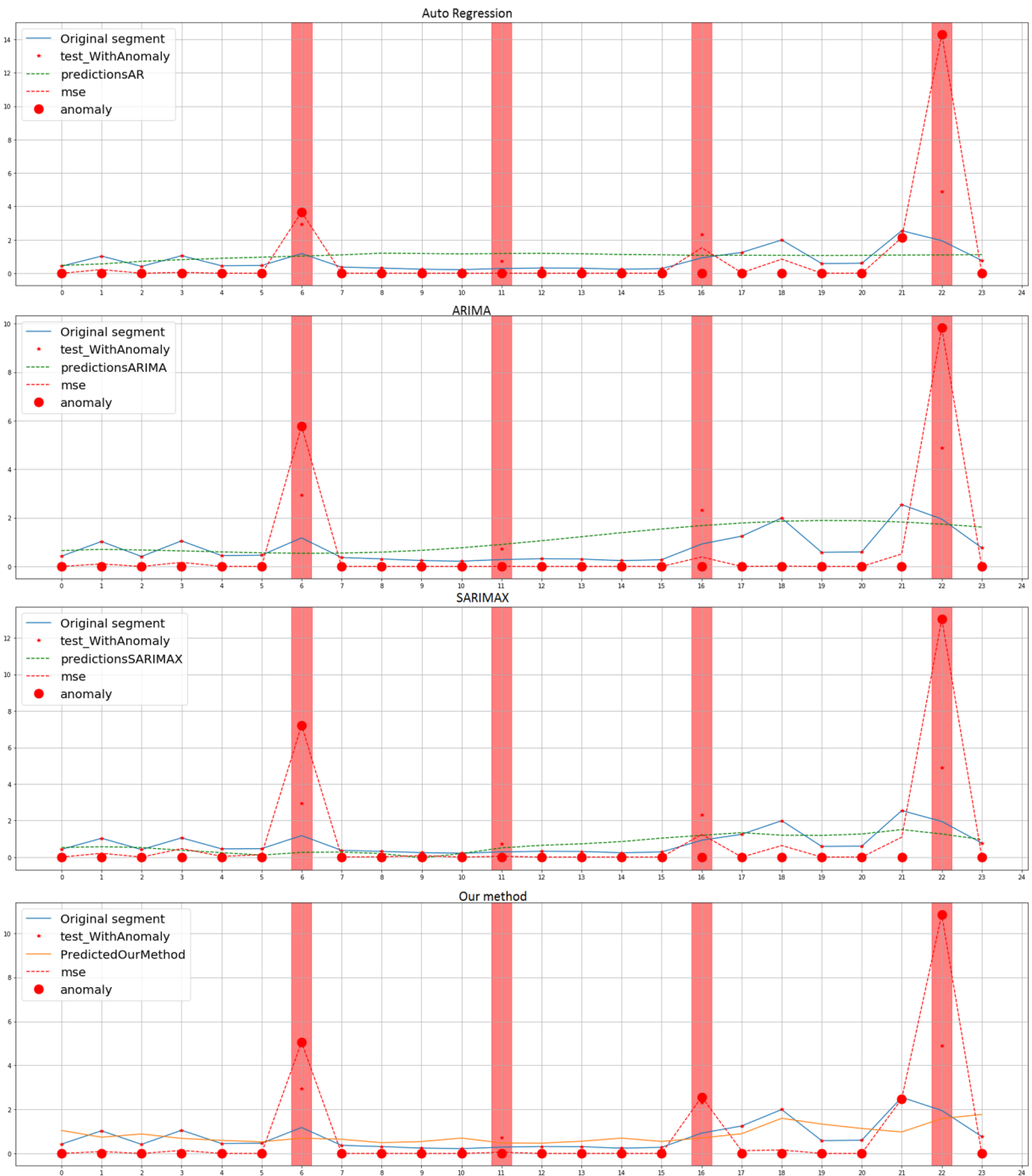
Fig. 17 The red shaded regions represent anomaly periods. Red stars represent the inserted anomalies. Red circles represent the detected anomalies. The red dash line is the mean square error between the predicted power consumption and the real power consumption
