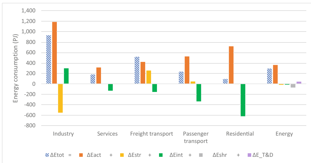
Fig. 2 Sectoral decomposition results from EEAS for changes in Canada’s total primary energy consumption between 1990 and 2013
