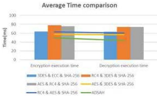
Figure 12. Average time comparison for encrypting and decrypting a file for the proposed model and the previous model.
