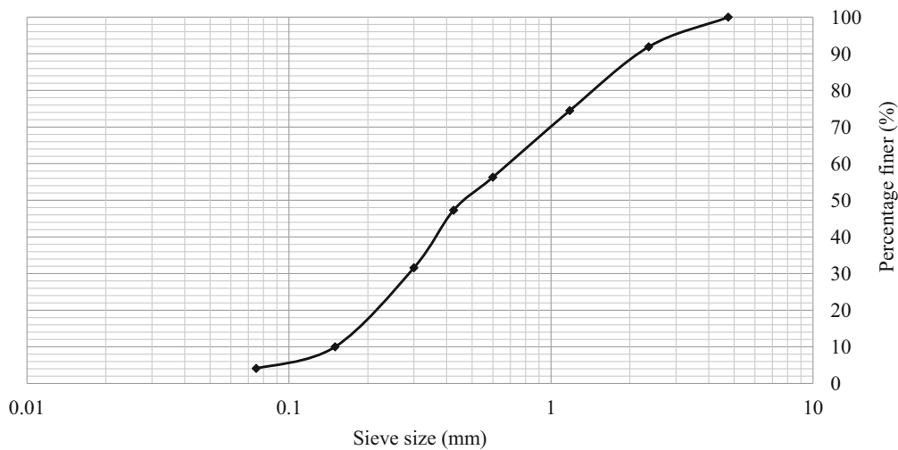
Figure 1. Particle size distribution curve of MSWI ash [20].
