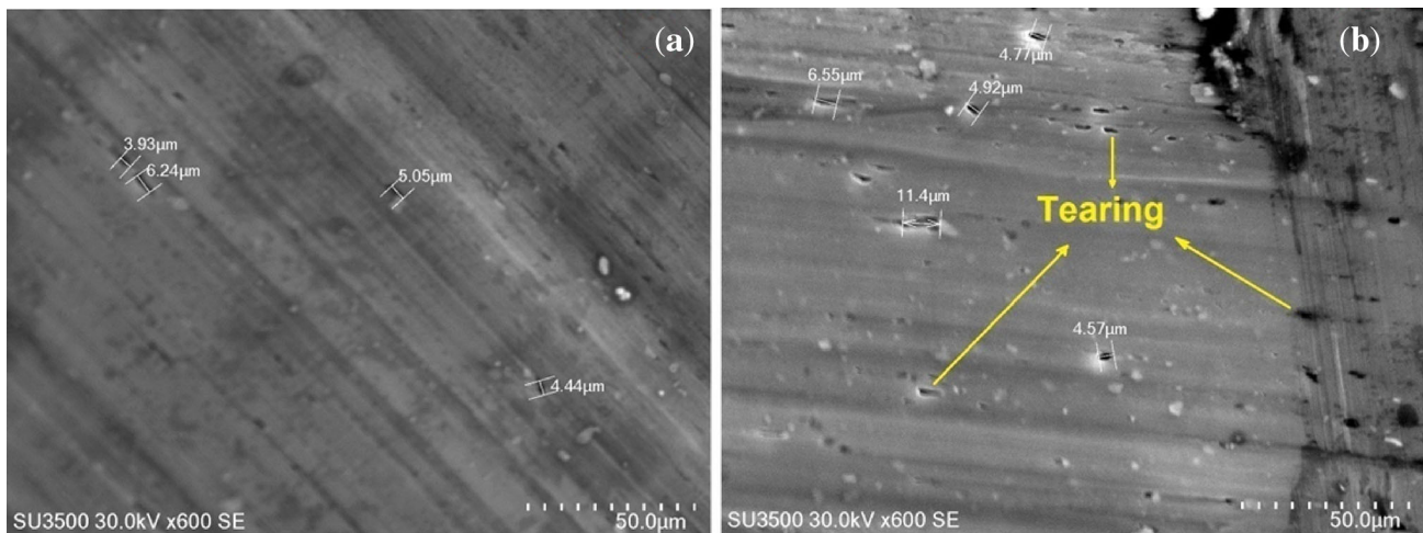
Figure 11. SEM images of chip underface showing the variation in ductile tearing at different velocity in case of machining with TiN coated tool, (a) at V_c = 336 m/min and (b) V_c = 540 m/min.
