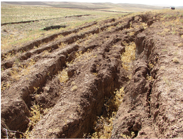
Figure 5. The elevated break lines with considerable opening at the border of subsidence band.
