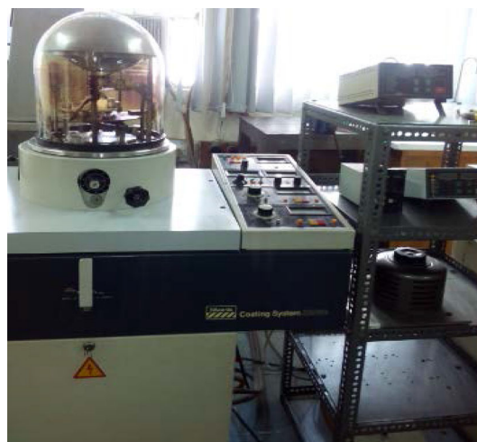
Figure 1. Preparation of ZnTe thin film. Sample using high vacuum coating unit (Edwards, U.K., and Model E306A).
