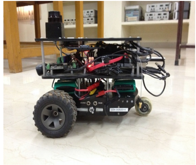
Figure 1. The Corobot CL2 mobile robot used for the experiment.
