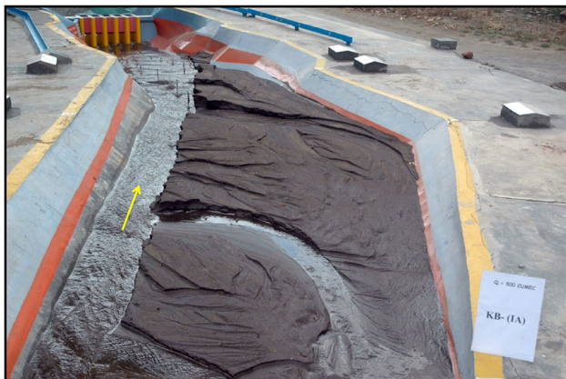
Figure 8. View of model near dam during flushing (Profile 1 and Q = 500 \text{ m}^3/\text{s} ).
