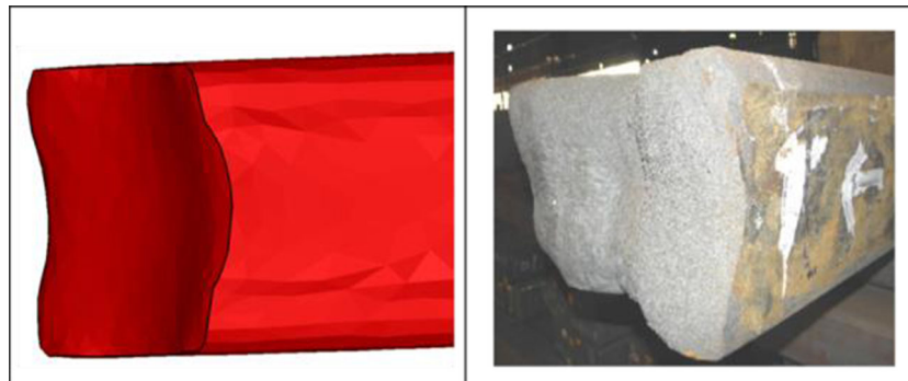
Figure 7. Comparison of the fish tail observed in simulation and actual experimentation after fourth pass of rolling using pass schedule (a) (roll groove with collar taper angle of 9^\circ , corner radius of 30 mm and groove depth of 63 mm).
