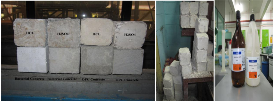
Figure 2. The appearance of specimens after immersion in 5% H_2SO_4 and 5% HCl.
