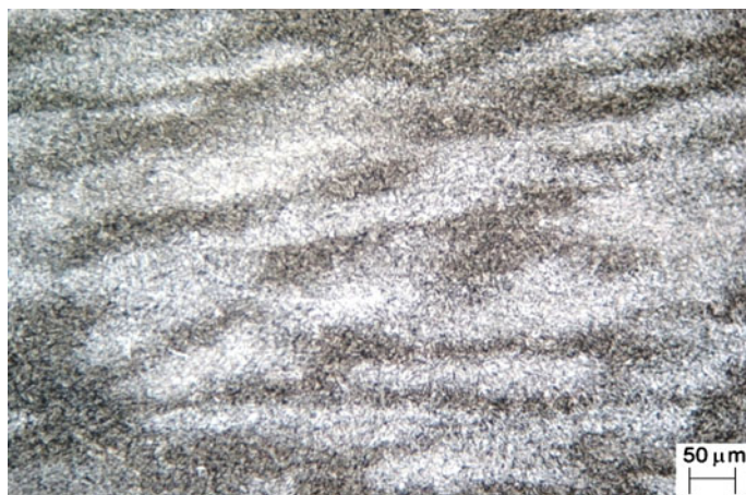
Figure 4. Optical micrograph showing microstructural banding induced by chemical segregation in H 1025 condition.
