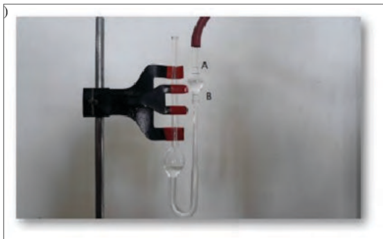
Figure 1. Ostwald viscometer (time taken by the liquid to flow between the two marks (A and B) was measured).
