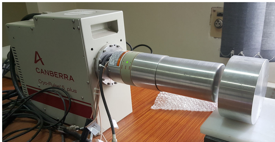
Figure 1. Aluminum cylindrical bowl set-up at IIT-Kanpur.
