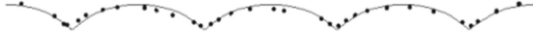
Figure 2. Trajectory of a tracer particle measured in a glycerol drop running down a superhydrophobic surface. The continuous line is a cycloid and the points are data from the experiments (adapted from [11] with permission).
