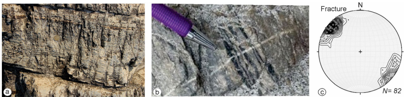
Figure 4. Extension fractures. (a) Termination of fractures at lithological boundaries. The fractures are at a high angle to the bedding surface. Camera facing NW. (b) Lack of shear offset in the bedding-parallel carbonate vein running across extension fractures. The carbonate vein is older than the fractures. Camera facing N. (c) Poles to extension fractures. Lower hemisphere equal-area projection (contours 2% per 1% area).
