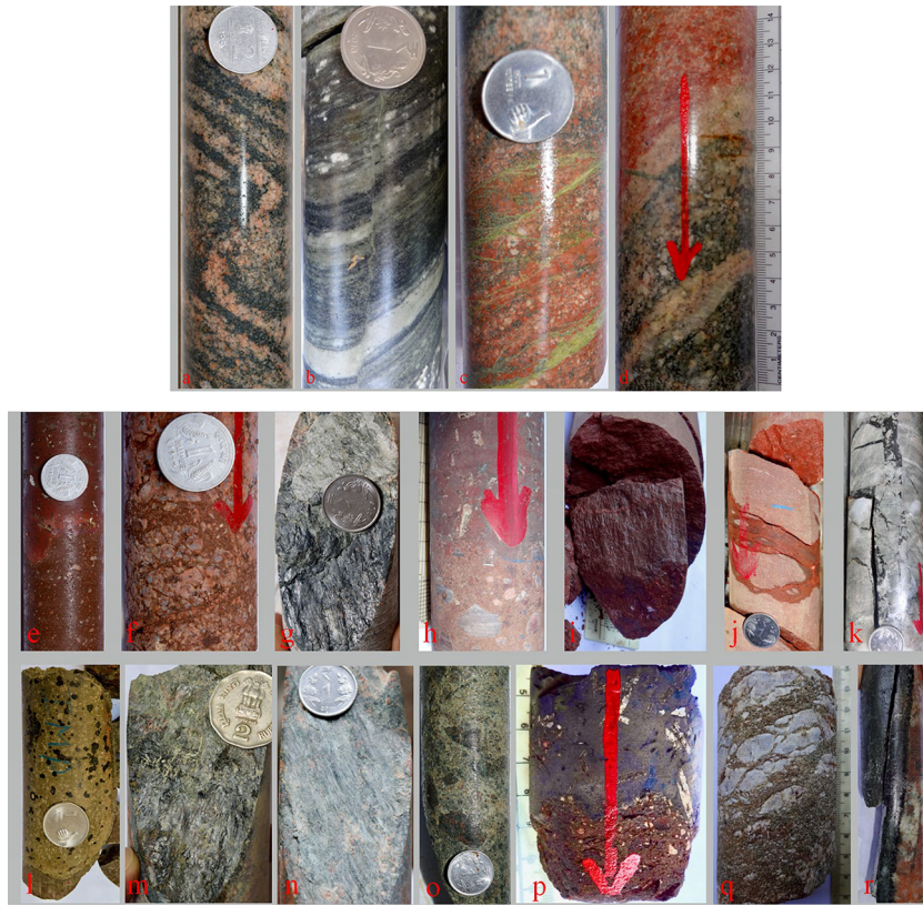
Figure 3. Photographs of borehole core samples from the Koyna seismogenic zone showing the sharp contacts between Deccan basalt and granitic basement rock at different sites and deformation signatures of ductile and brittle nature preserved in the granitic basement rock. (a) Core sample from KBH-1 at 1060.00 m depth representative of S_{1-2} segregated bandings within quartzofeldspathic gneiss. (b) Core sample from KBH-5 at 857.40 m depth showing segregated layerings, which are mainly S_{1-2} fabrics. A near-vertical fault surface displacing S_{1-2} fabrics along which secondary precipitations are found. (c) Core sample is from KBH-6 at 805.75 m depth exhibiting the same S_{1-2} fabrics within granite gneiss. Interconnected fractures mostly follow the S_{1-2} fabrics orientation. These fractures are filled up with secondary siliceous precipitations. (d) Core sample from KBH-7 at 1346.25 m depth representing interlayerings of granite and quartzofeldspathic gneisses with prominent S_{1-2} fabrics. (e) Core sample showing sharp contact between Deccan basalt and the underlying granite at 932.5 m depth in borehole KBH-1. Plagioclase laths are prominent within Deccan basalt in the upper portion, while clasts of quartzofeldspathic aggregates are entrapped within the weathered surficial part of granite in the lower part of the sample. (f) Core sample collected from 936 m depth in borehole KBH-1 showing anastomosing fractures and ferruginous secondary precipitations. (g) Core sample collected from 1159 m depth in borehole KBH-1 showing a fault surface containing down-dip slickenlines on a slickenside. (h) Core sample showing the sharp contact between Deccan basalt and underlying granitic basement rock at 499.70 m depth in borehole KBH-5. Plagioclase laths are present within Deccan basalt in the upper part of the sample, whereas large quartzofeldspathic clasts entrapped within fine matrix are present in the lower part. (i) Core sample from 500.50 m depth in borehole KBH-5 showing prominent down-dip slickenlines on a well-developed vertical fault surface. (j) Core sample of sheared granite-gneiss from 500.85 m depth in borehole KBH-5, showing lensoid clasts of host rock entrapped within fine-grained gouge matrix of same material within a fractured zone. (k) Core sample from 732.00 m depth in borehole KBH-5 showing a near-vertical master fault with associated tensile fractures. A narrow fault zone with brecciated angular fragments of host rock is seen. Angular clasts of host rock are entrapped within fine-grained gouge matrix. The dark black portions along these fractures represent extremely fine grained, pseudotachylite melts injected from the master fault into the associated tensile fractures. (l) Core sample showing the sharp contact between Deccan basalt and the underlying granitic basement rock at 775.04 m depth in borehole KBH-6. The basement rock below this contact is highly fractured and shattered. (m) Core sample from 897.60 m depth in borehole KBH-6 showing a thin layer of pseudotachylite along the fault surface. Down-dip slickenlines are prominently seen on this fault surface. (n) Core sample of a fault surface at 948.50 m depth in borehole KBH-6 showing a slickenside with prominently developed slickenlines that formed due to friction during movement. (o) Core sample showing highly fractured and brecciated granite rock at 1044.75 m depth in borehole KBH-6. Fragmented clasts of host rock are entrapped within fine matrix of gouge material. Anastomosing fracture network filled with greenish silicification from channelized water is also observed. (p) Core sample showing the direct contact of Deccan basalt and the underlying granitic basement rock at 1251.23 m depth in borehole KBH-7. Plagioclase laths are seen in the first basaltic flow. (q) Core sample from 1253.72 m depth in borehole KBH-7 showing fractured quartzofeldspathic layers within granite gneiss. Fractures are filled up with ferruginous precipitations. The mafic layers are mostly weathered and altered in this section. (r) Core sample from 1476.70 m depth in borehole KBH-7 showing a mafic dyke (amphibolite) body in a near-vertical orientation and having direct contact with the basement rock.
