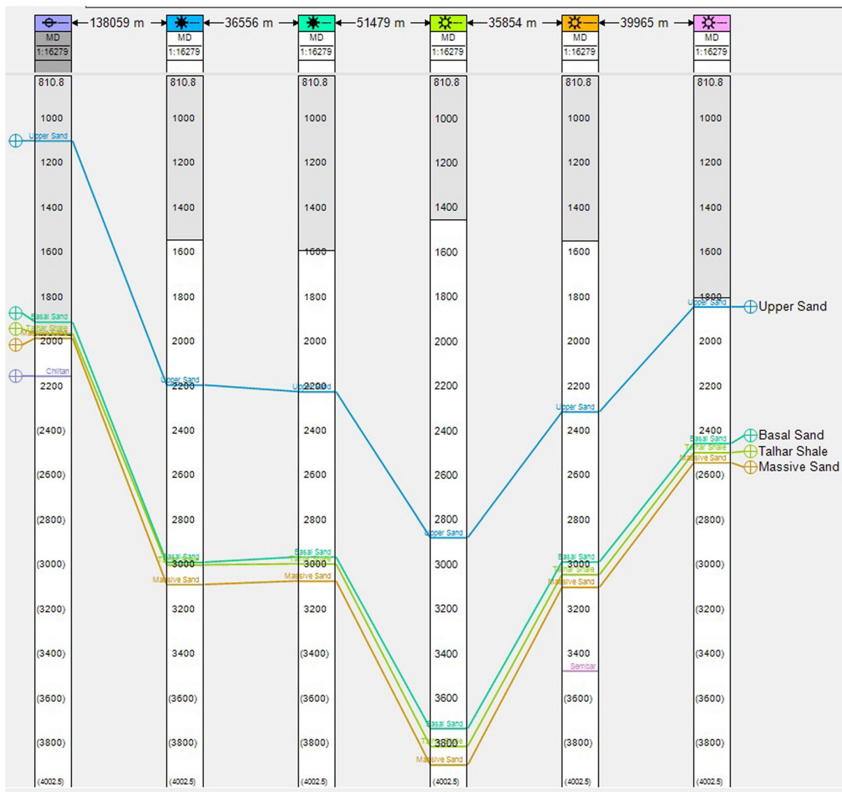
Figure 14. Well correlations for Lower Goru facies distribution along the cross-section X-Y (figure 1) in the Southern Lower Indus basin of Pakistan.
