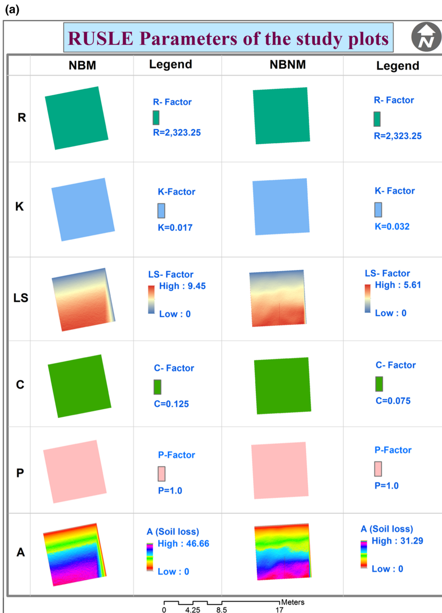
Figure 4. (a, b and c) Soil loss per year and RUSLE parameters for different plots.
