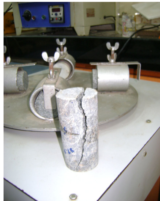
Figure 4. Fracture developed after UCS test.
