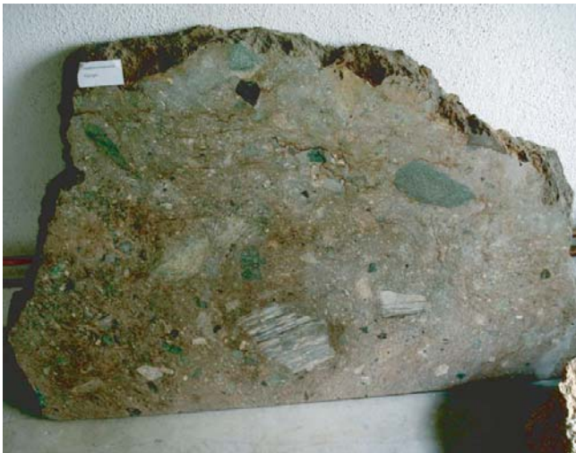
Figure 6. Impact melt breccia from Pölsingen, Ries crater. This sample displays a polymict population of target rock clasts set into a finest-grained crystalline melt matrix (Courtesy ZERIN, Nördlingen). Slab about 1 m in width.
