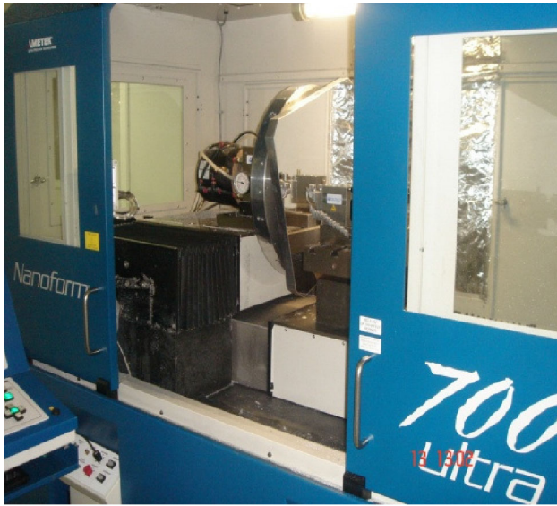
Figure 3. A finished mirror facet for the MACE telescope on DTM.
