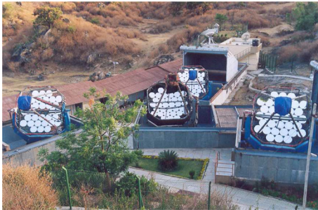
Figure 2. The TACTIC telescope array at GOALS, Mount Abu. The central element of the array is used as a single IACT for the GeV–TeV \gamma -ray observations.
