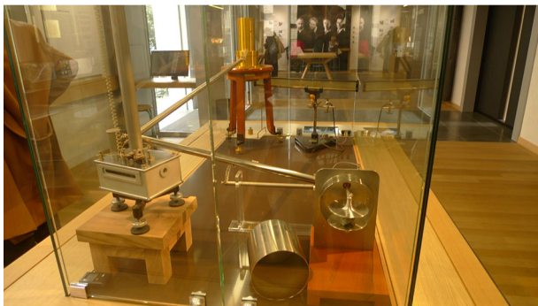
Figure 8. The electrometer which the Curies used to measure radioactivity by ionizing the gases with the emitted radioactivity. The instrument is kept at the Musée Curie, Paris, France (Photo: S.L.).
