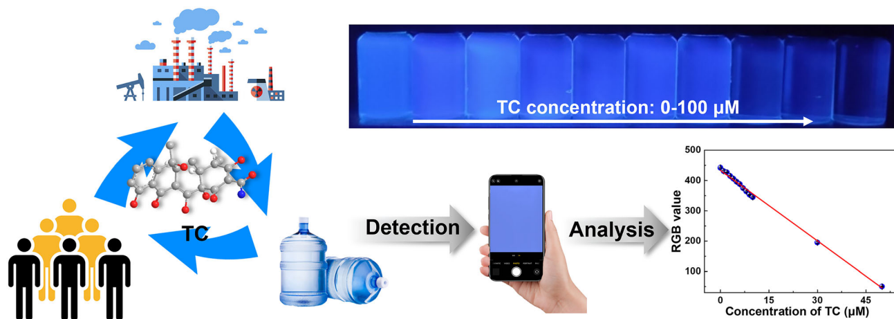
Figure 6. Schematic diagram of TC residue detection in real sample by smartphone sensing platform.
