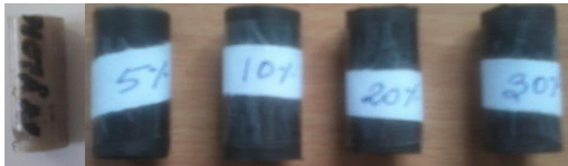
Figure 4. PA6 and PA6 with graphite test specimens.
