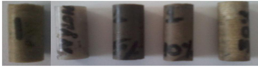
Figure 3. PA6 and PA6 with Al 2 O 3 test specimens.
