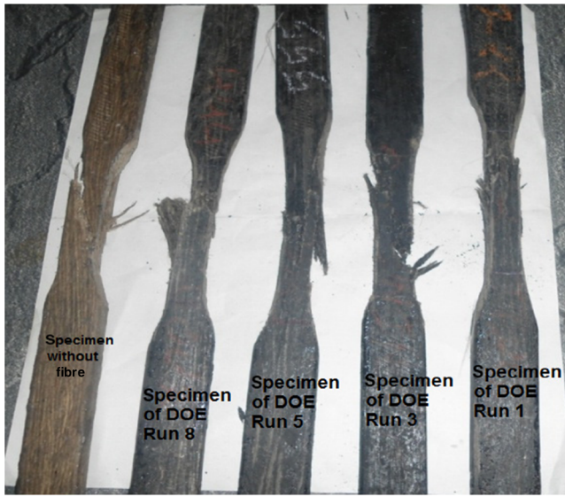
Figure 5. JFRP composite tensile test specimen after tensile test.
