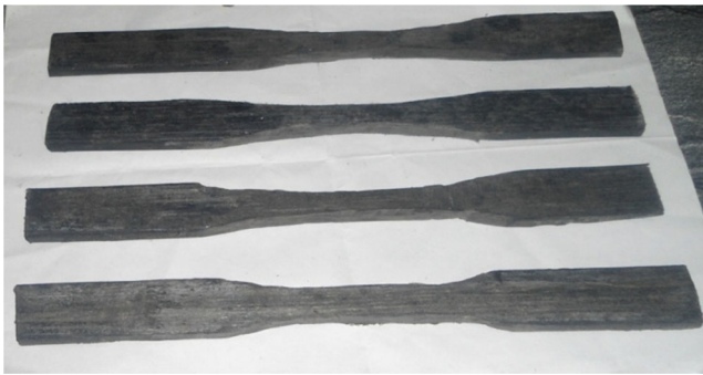
Figure 3. GFRP composite tensile test specimen according to ASTM D638.
