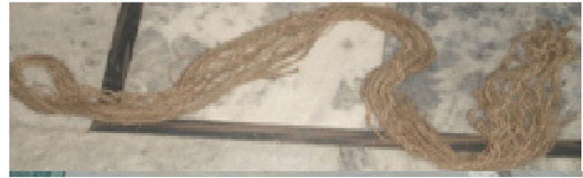
Figure 2. Fibre bundle for pultrusion.
