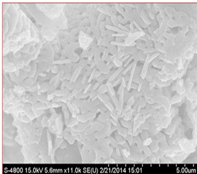
Figure 2. SEM pattern for combustion synthesized \text{LiBaPO}_4:\text{Tb}^{3+} phosphor.
