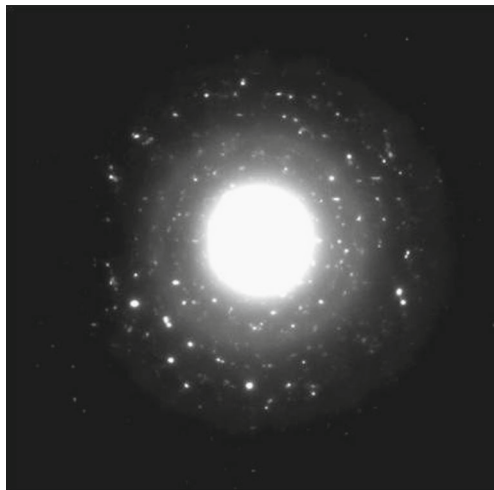
Figure 2. Selected area diffraction pattern of boron specimen, synthesized by electrowinning at a temperature of 1073 K by applying a potential of 4.5 V on a mild steel substrate for 6 h.
